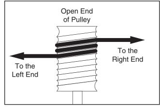
Figure 18. Cable orientation on pulley.
